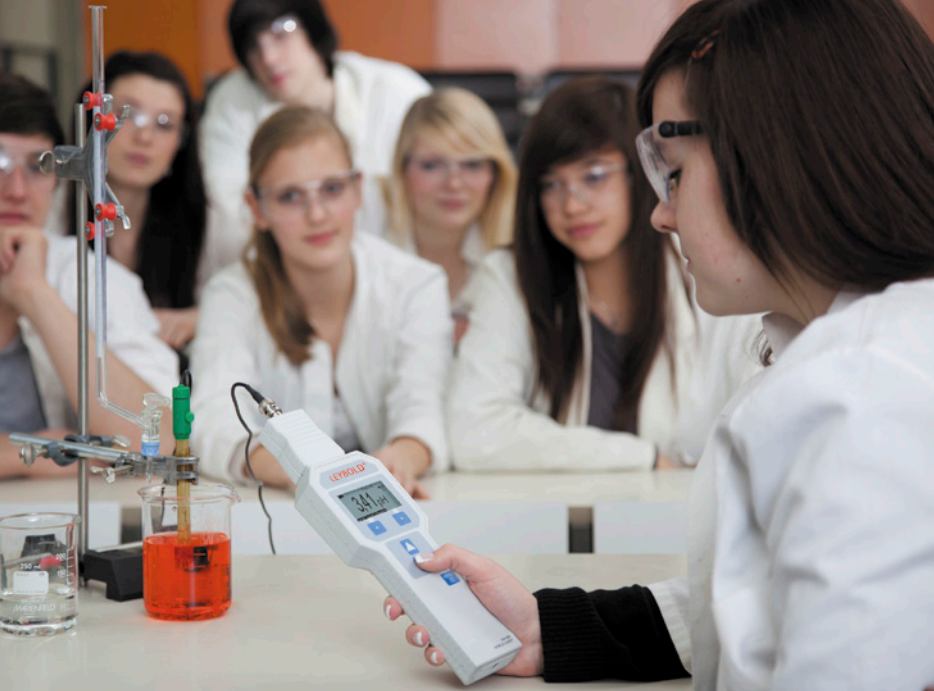
Monitoring of the pH value during a titration with Mobile-CASSY
